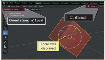
If more than one object is selected when using the *Local* axes for scaling, the *Scaling* gizmo displays the *Local* axes of the *active object*.
