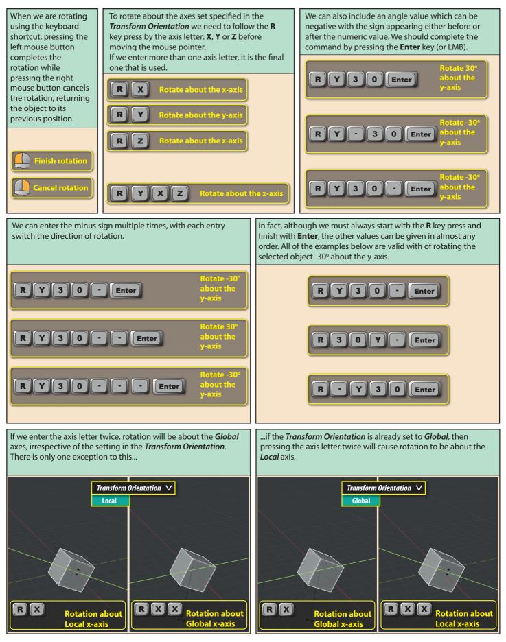
**Trackball Rotation** gives free rotation about all three axes and is initiated by pressing **R** twice. Rotation follows the position of the mouse pointer.
